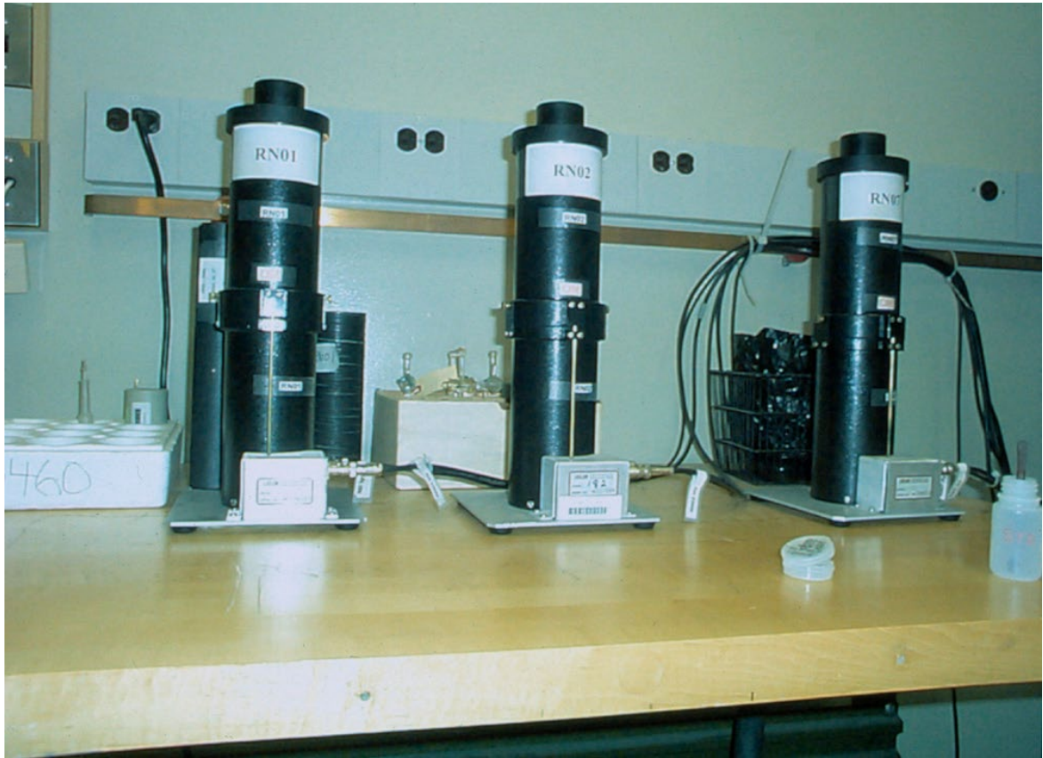
Computer controlled counters for alpha scintillation cells
