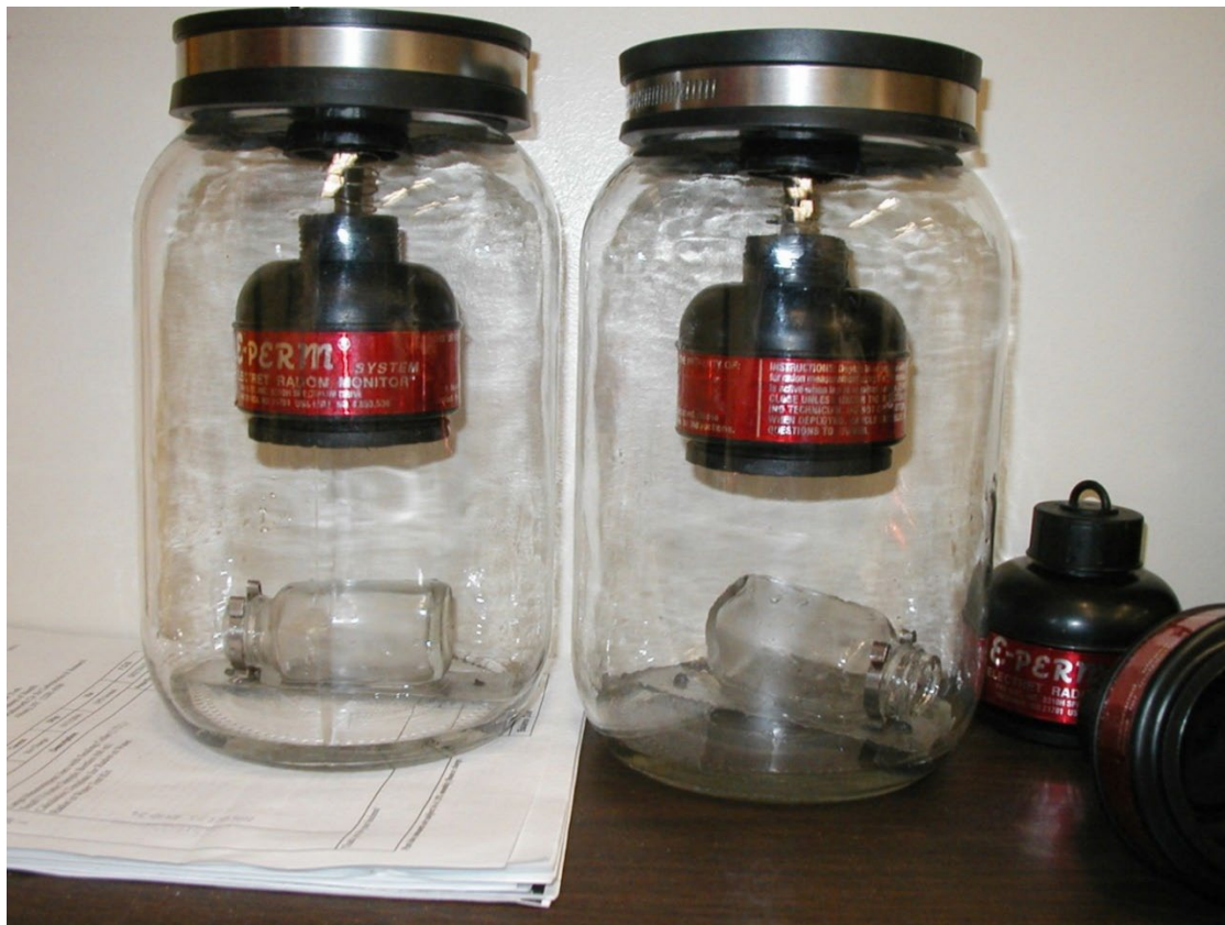
Measurement using electret method Kitto, J. Environ. Radioact. 99, 1255-1257 (2008)
