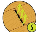
6 Gaps in suspended floors
