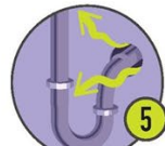
5 Gaps around service pipes
