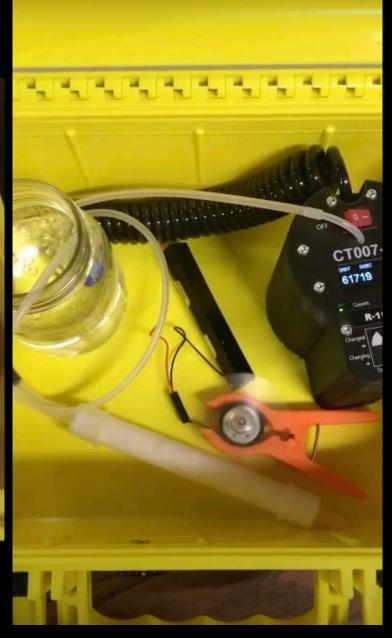
Without bubbling air through the sample the air concentration in the case levels out at around 275 pCi/L.
