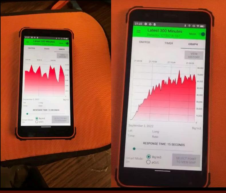
With bubbling air through the water sample, the air concentration in the case levels out at around 1700 pCi/L in about 10 minutes.
