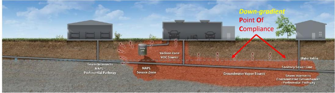
Point of Compliance (POC) in 'deep-native' soil gas <u>only subject to diffusive flow</u>, and away from Human-built subsurface structures that could induce advective flow & form locally-reduced conc.
