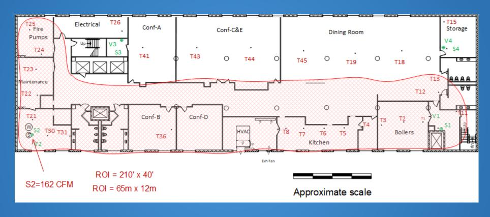
S2 airflow 162 CFM S1 airflow 141 CFM 8" Baseline only 0.28" SP - S1 0.52" SP
