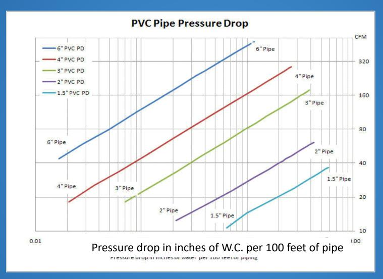
Derived from 30 & 60 foot lengths of piping tested
