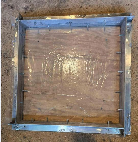
Aluminum frame box with  $\frac{3}{4}$ " plywood to create an air space
