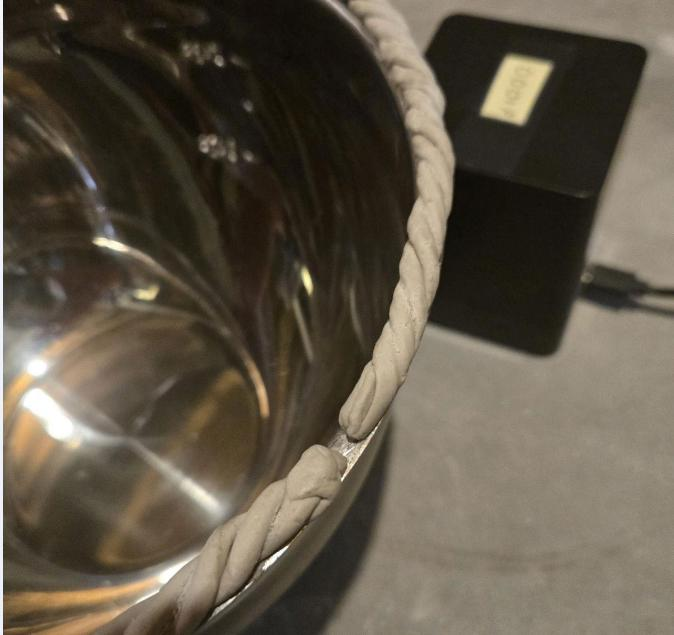
Twist three strands of Mortite into a rope. Hand compress onto edge. Leave space for Elec cord and compressed air
