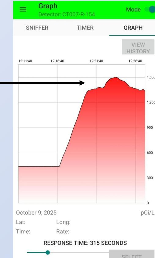
**Consistent Flux of about 23 pCi/SqFt/Hour out of the slab**
