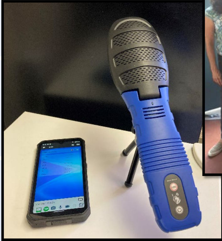
Indoor Air Sensor – VOC, CO 2 ,CO
