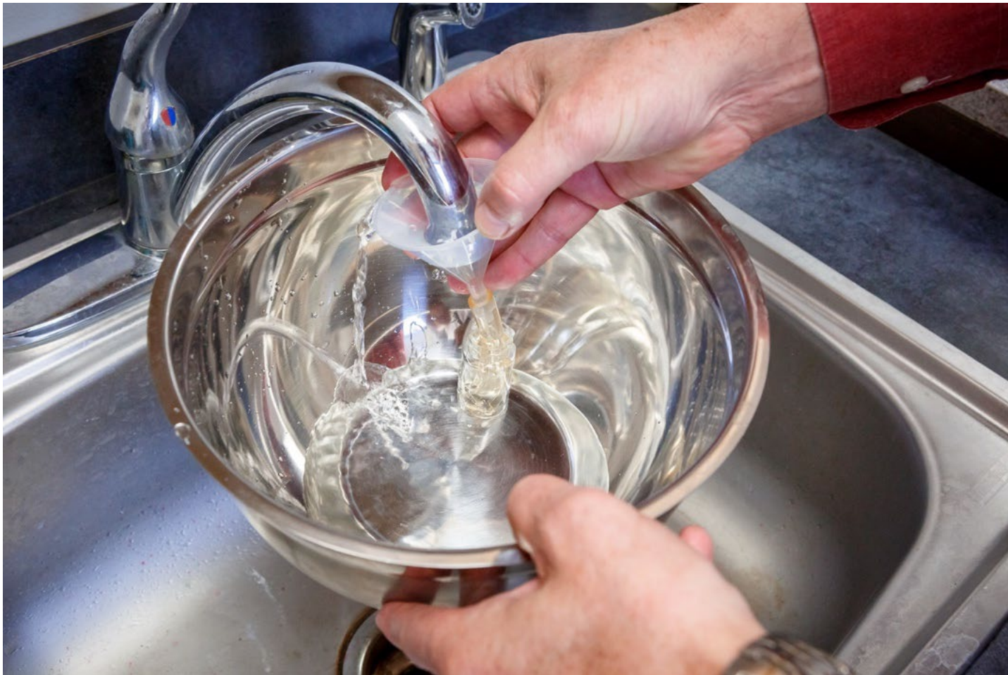
Upright funnel— Immersed bottle method
